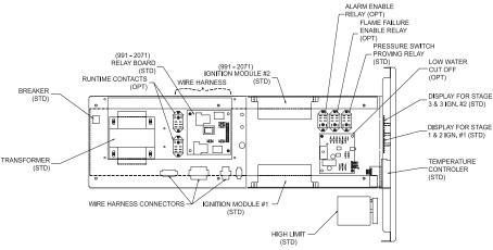
FIG. 33 Control Panel Component Location Drawing
